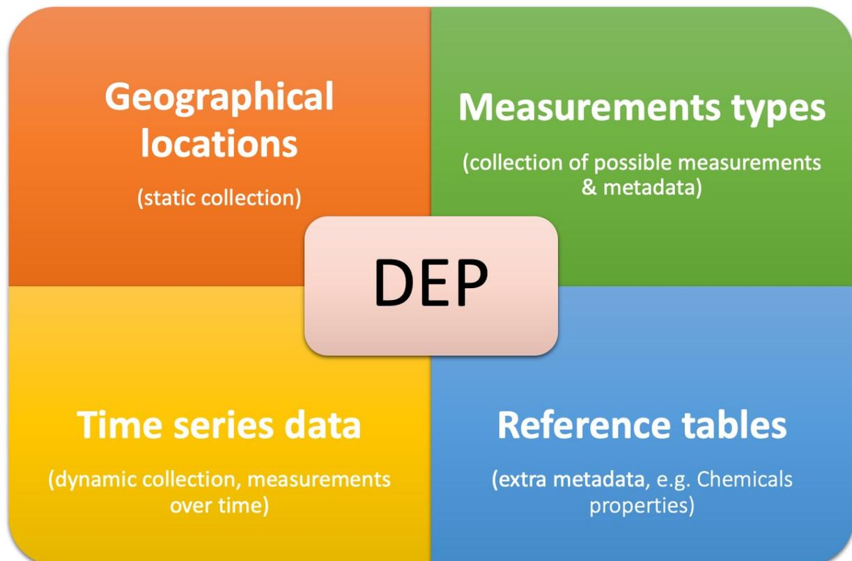
The files formatted according to the DEP can be directly parsed into the unified MongoDB storage solution. The DEP is composed of 4 parts, one specifically devoted to one kind of data or other pieces of information. Geographical information and time series data make the core of the DEP, and are represented with two CSV files: *LOCATIONS\_META* and *TS\_DATA*.
