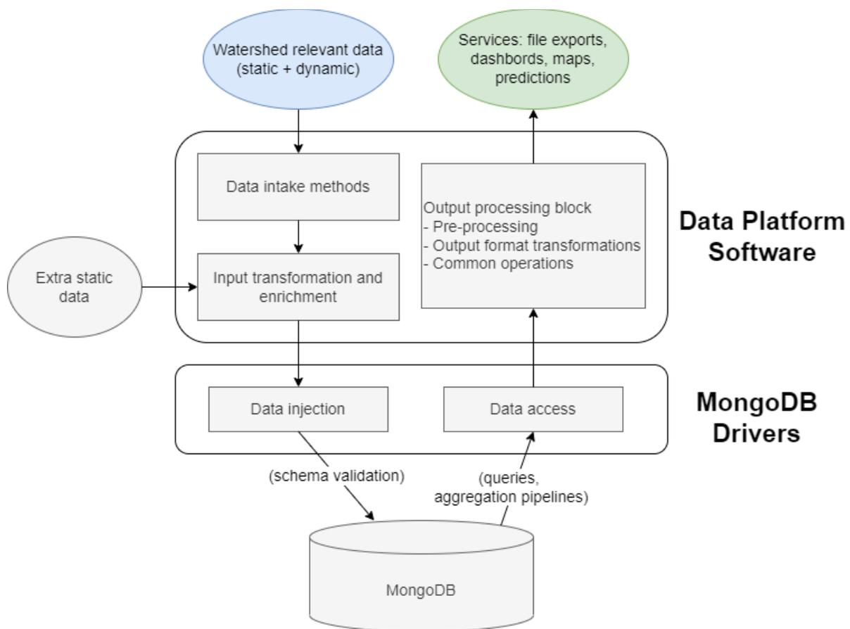
On the left, we follow the input data processing and injection in the DB.
